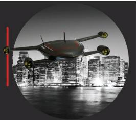
It is a HSVSTOL unmanned aerial vehicle capable of carrying out multi-mission in the civil and military fields, operating under low or at high flight speeds due to its versatile propulsion options – Turbofan, propeller or EDF.
