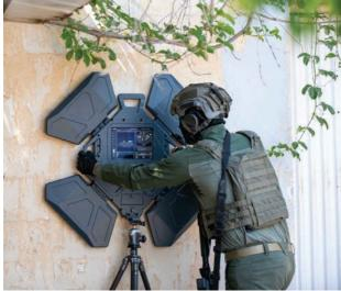
The Xaver™1000, the new generation of the Camero-tech>s Xaver™ product line, is a real-time 3D 'Sense Through Wall' imaging radar equipped with an innovative Al-based tracking algorithm of dynamic/static target patterns behind walls in more than 30 meters.
